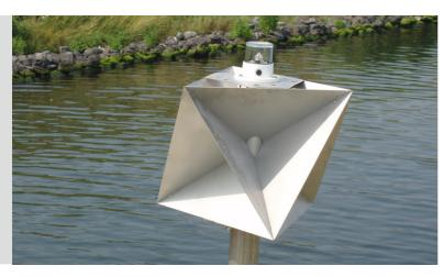
The IML 85 AL LED is a compact signal lantern with a single, high intensity LED light source. The light output can be programmed by infrared remote control. The base comprises marine grade aluminium, coated with two layers of high impact epoxy. The colour is the same as the emitted light. A membrane is incorporated for air pressure equalisation and to prevent moisture from entering the casing.
